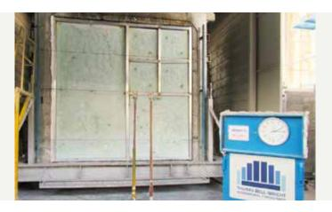
The picture presents the specient view after the 120 minutes test where performed. The photo was taken on the unexposed side.
