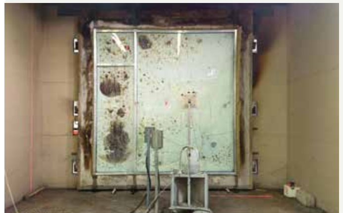
The photo shows the specimen after the 60-minute test was finished. View from the unexposed side.
