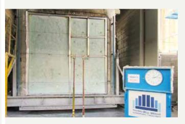
The picture presents the specient view after the 120 minutes test where performed. The photo was taken on the unexposed side.
