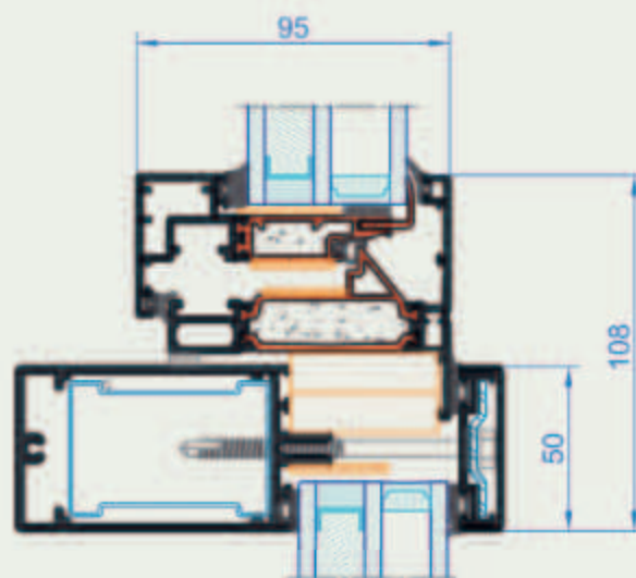
Facade window (example with facade AW50)
