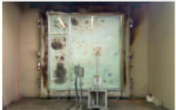
The photo shows the specimen after the 60-minute test was finished. View from the unexposed side.
