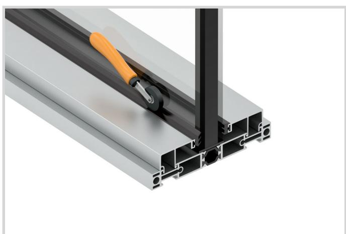
6.5 - Ensure that the gaskets fit tightly, by cutting the gaskets in a 45 degree angle in the corners.
