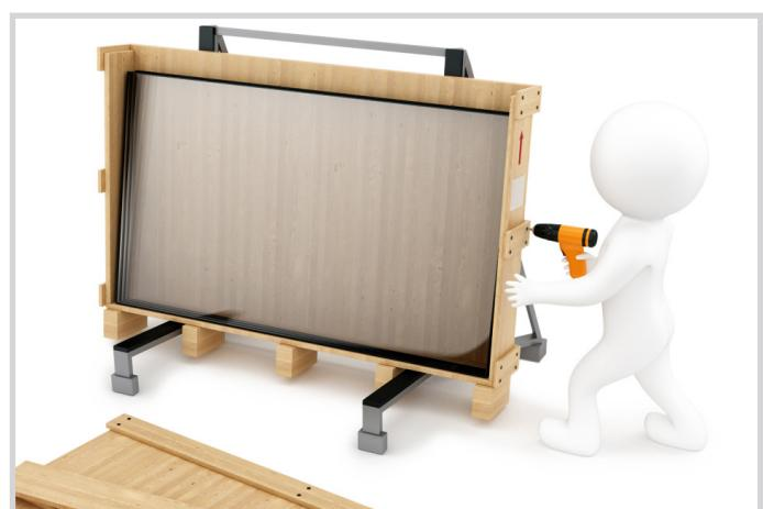
5.2 - Unpack the glazing and prepare to lift the glass into position. Never put the glass directly onto the floor as it can cause the glass to collapse. Always elevate the glass from the floor using either planks of wood or other suitable material.
