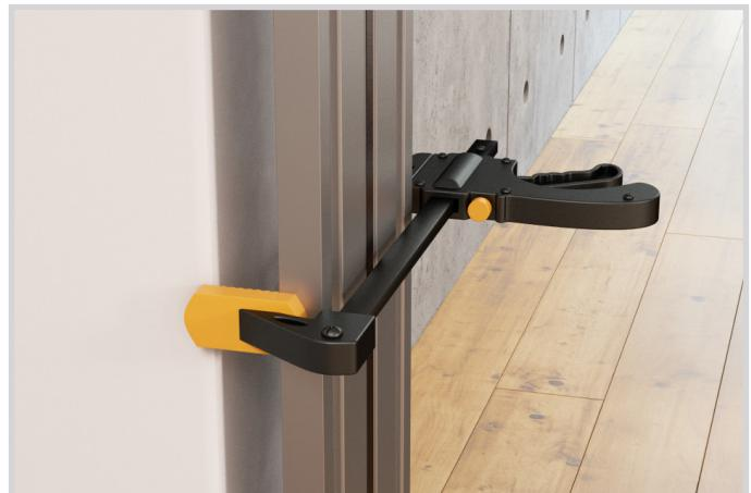
3.1 - Put the frame into the designated hole and fasten it temporarily with clamps and the positioning bolts are completely tightened. Make sure not to tighten the bolts too hard, as it can damage the frame.
